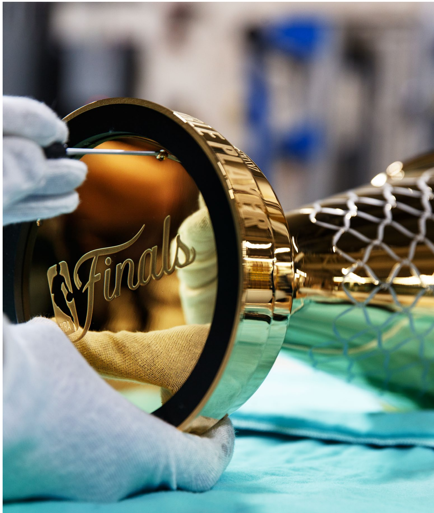
A silversmith attaches the reflector plate to the NBA Bill Russell MVP Trophy.
