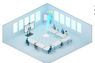
Automatic, dynamic beamforming technology ensures that a speaker is clearly audible, no matter where they move in a room
