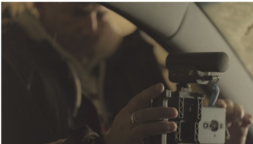
Rayner’s choice to use the MKE 400 means that one connector has been removed, as monitoring is provided onboard via a 3.5-mm jack connector
