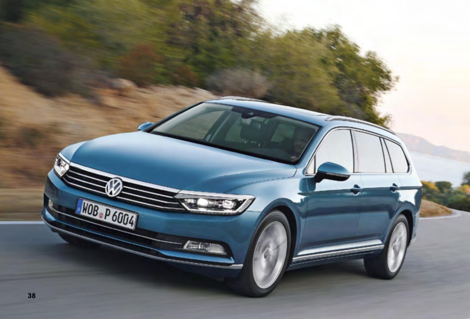
the wide indicators (twelve LEDs) emphasise the headlight's design. LEDs for the static cornering light are also positioned on the inner side of the headlight.
