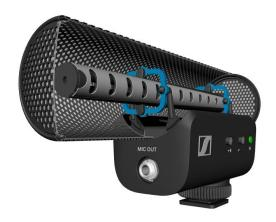
A look inside the MKE 400 reveals the acoustic interference tube, which is shock-mounted (blue elements) to prevent handling noise from transferring to the capsule. The mic housing doubles as a standard windscreen, saving space and hassle.
