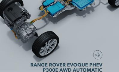
1.5-litre three-cylinder Ingenium Petrol 309PS (227kW) / 540Nm 0-60mph - 6.1s 0-100km/h - 6.4s
