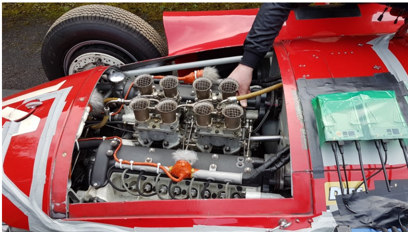
To the right, two Sennheiser EK 6042 receivers mounted to the Lancia-Ferrari D50A, receiving audio from large-diaphragm mics made wireless by SKP plug-on transmitters
