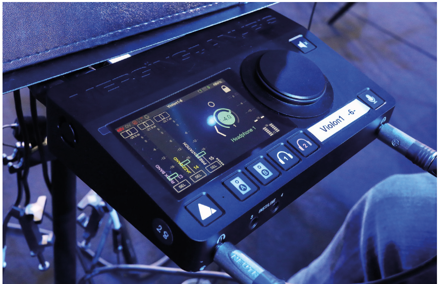
Interface in the personal mixer mode for violinists Here, for example, users can adjust the stem components for rock band, jazz band and presenter
