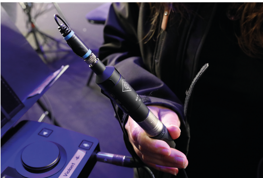
MCM-100 output stage in wired operation. If necessary, the jack connection can be fixed using a clip supplied, otherwise it releases under tension to prevent damage of instruments through falling if someone stands up and forgets the wiring
