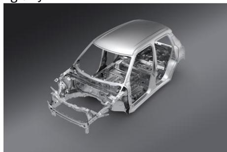
A comprehensive overhaul of the underbody’s structure and component layout has resulted in the replacement of the segmented frame of the previous platform with a continuous frame that increases underbody stiffness. The new frame is characterised by a smooth, curving form that efficiently disperses energy, enhancing collision safety. Overall body rigidity has been further improved with an increase in spot welds, improving steering-yaw rate linearity and control.
