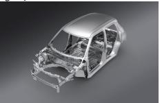
A comprehensive overhaul of the underbody's structure and component layout has resulted in the replacement of the segmented frame of the previous platform with a continuous frame that increases underbody stiffness. The new frame is characterised by a smooth, curving form that efficiently disperses energy, enhancing collision safety. Overall body rigidity has been further improved with an increase in spot welds, improving steering-yaw rate linearity and control.
