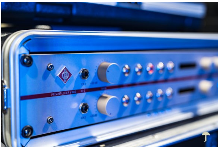
The Neumann V 402 was looped in between the wireless system and the mixing desk
