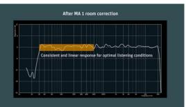
By the way, the MA 1 system also ensures that Neumann speakers of different sizes reproduce audio material consistently. From the small KH 80 DSP, through the KH 150 available at the StrandGut Resort, to the large KH 420 model (with DSP sub), automatic monitor alignment achieves a homogenous sound playback. While the reproduction of deep frequencies naturally varies (casually put: bigger = deeper bass), the overall sound characteristic remains perfectly comparable.
