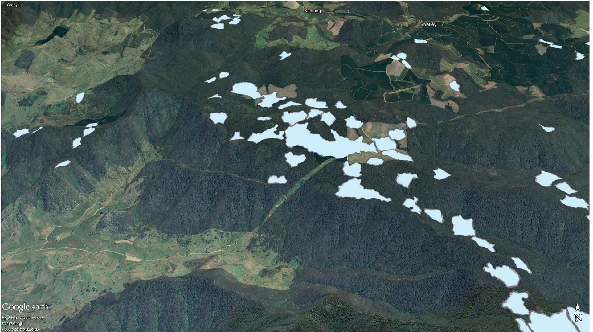
*Figure 11: Potential PHES upper reservoir sites near the Tallangatta Valley (Victoria) The easement corridor for the 330 kV transmission line can be seen in this image.*
