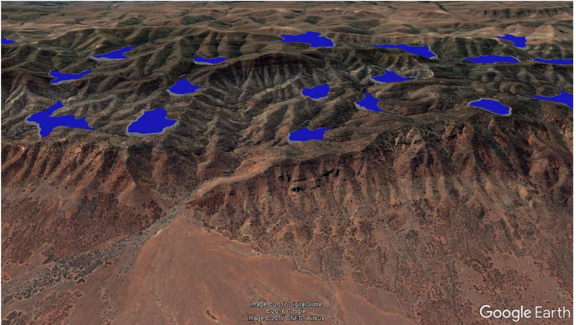
*Figure 6: Potential PHES upper reservoir sites in Region A, east of Port Augusta. The lower reservoirs would be at the western foot of the hills (bottom of the image).*
