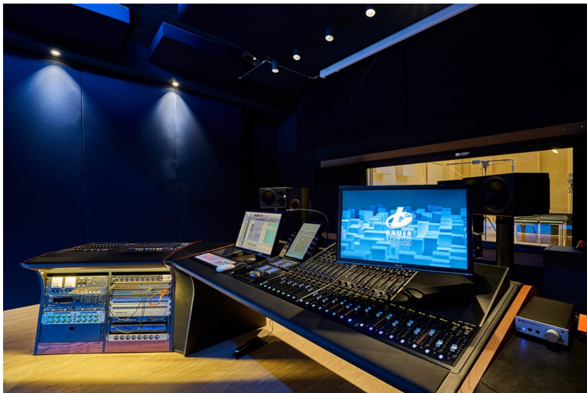
The redesigned Studio 2 is equipped with an Avid S6 console, which also serves as the monitor controller for the 5.1.4 or 7.1.4 setup. (Photo: Bauer Studios)
