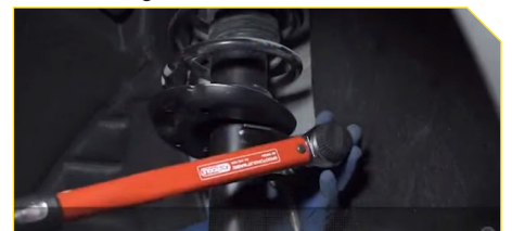
14. Screw the anti-roll bar rod upper nut and tighten to 65Nm
