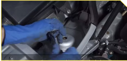
6. Unscrew the indicated screws of the top mount
