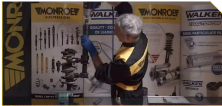
7. Install the spring compressor to unscrew upper retaining nut
