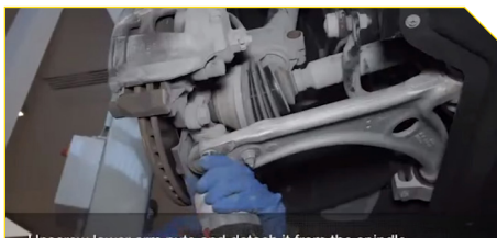
4. Unscrew the indicated screws of the bottom mount
