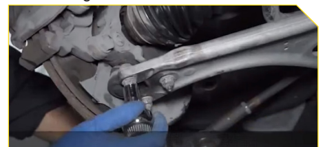
13. Fit the lower arm and tighten the retaining nuts to 100Nm
