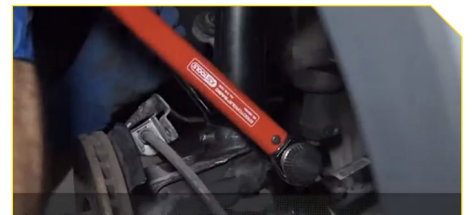
12. Tighten the retain bolt of the steering knuckle to 70Nm + 90°
