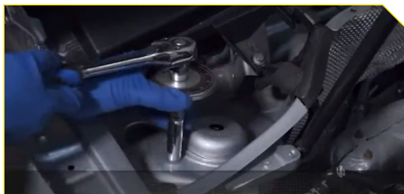
10. Fit the upper mounting retaining screws and tighten to 15Nm + 90°
