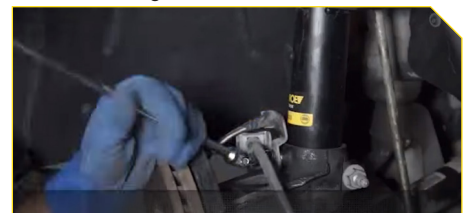
15. Fit the brake piping bracket retaining screw
