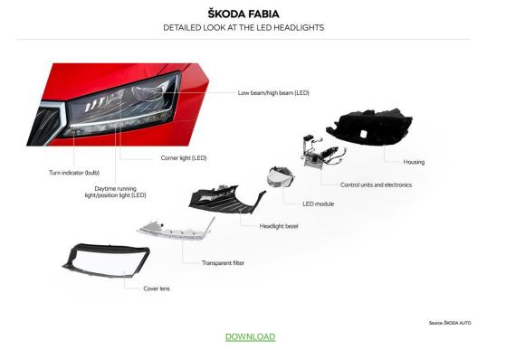
The new LED headlights are significantly brighter yet use less energy and have a longer lifespan. One LED is used for dipped beam and high beam, whilst a second one is used for illuminating corners. Four other LEDs are used for daytime running lights and parking lights. The dipped beam of the new system emits 66% more light than the previous top-of-the-range version. This means the LED headlights clearly outperform the currently brightest headlights.
