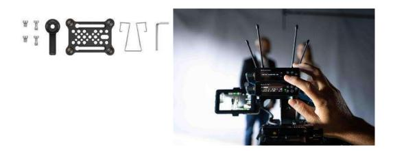
EW-DP's magnetic plate allows filmmakers to simply (and securely) stack multiple receivers. Alternatively, the plate can be used with the provided clip to wear the receiver on the belt or attach it to the sound bag
