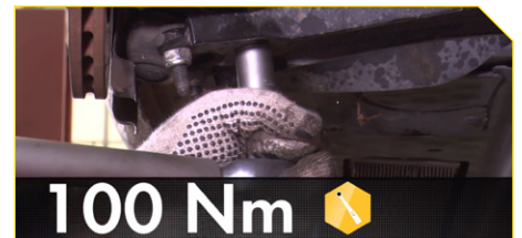
12. Fit the lower track control arm to steering knuckle and tighten to 100Nm
