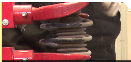
5. Install the spring compressor to unscrew upper retaining nuts
