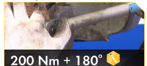
14. Tighten steering knuckle mounting screw half-shaft to 200Nm + 180°
