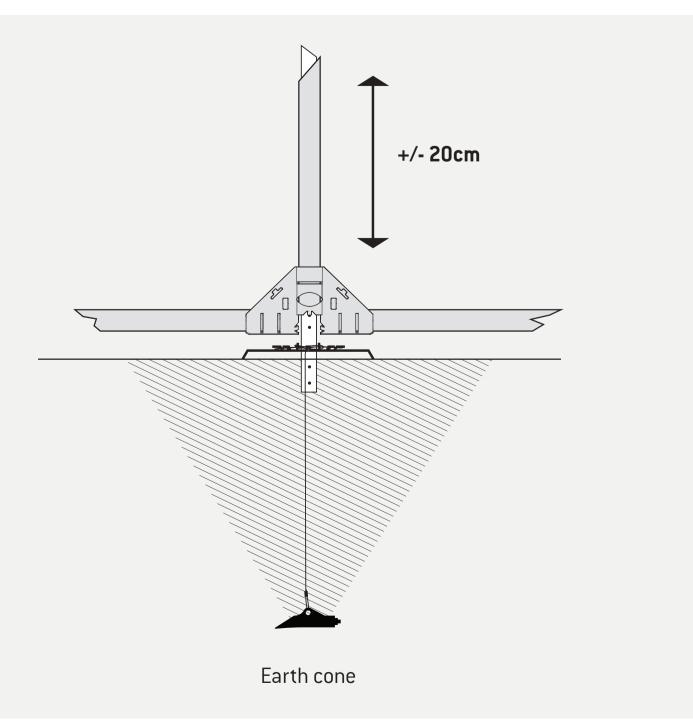
THE GROUND ANCHORING SYSTEM is design to fit various ground conditions, from grabble and sand and clay to asphalt. The anchor is height adjustable, which allows the shelter to be built on uneven grounds or in slopes of up to 7 degrees. The concept involves a specially designed anchor which is driven and locked into the ground with a driver - no digging is required to lock it into position.
