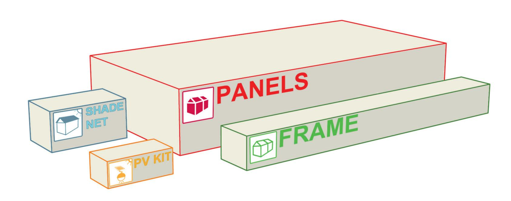
PACKING The Refugee Housing Unit is packaged in four separate packages which can be combined or used indecently in order to respond to the shifting needs and budgets of relief operations. The total target weigh of the Shelter is 98 KG and the packing volume is 1.5 cubic meters. All packages can be carried by two people.
