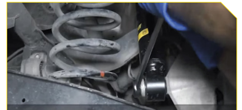
11. Tightening lower mounting screw to 180Nm
