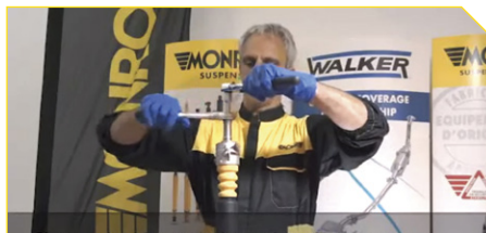
8. Replace shock absorber and its components with new ones and tighten top mounting nut to 25Nm
