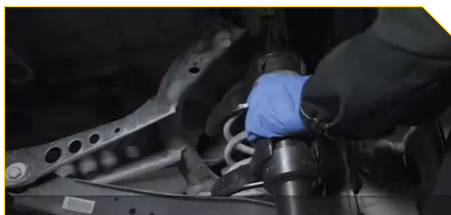
4. Install the spring compressor and compress the spring
