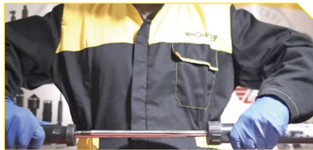
7. Compare the old shock absorber to the new one to be sure it fits
