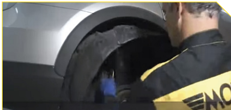
3. Remove the wheel arch protection shield
