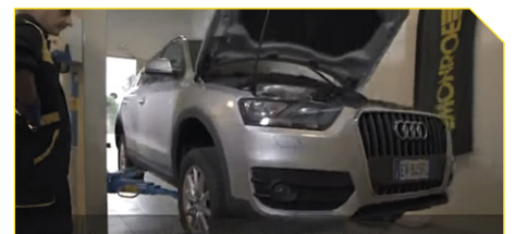
13. Lower the car and tighten wheel nuts to 140Nm
