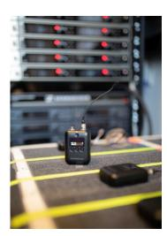
The SK 6212 mini-bodypack transmitter impresses with compact dimensions and an operating time of 12 hours
