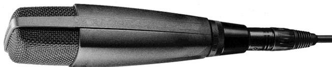
Thanks to its large diaphragm, the MD 421-II has a wide, condenser-like frequency response of 30 – 17,000 Hz. It is fitted with a five-position bass roll-off switch (from M for music to S for speech), which helps to compensate for the proximity effect where needed and reduces impact sound. The filter can also be dialled in if you prefer to place an emphasis on the higher
