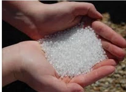
Master batches with different additives and pigments
