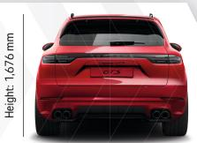
Front gauge: 1,682 mm Rear gauge: 1,665 mm
