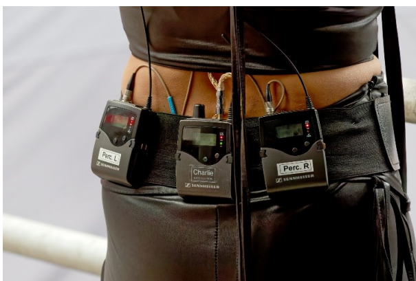
Multi-instrumentalist Charlie Klauser wore as many as three beltpacks: an in-ear receiver as well as two SK 500 transmitters, which transmitted the percussion signals from Sennheiser MKE 2 clip-on microphones attached to her hands
