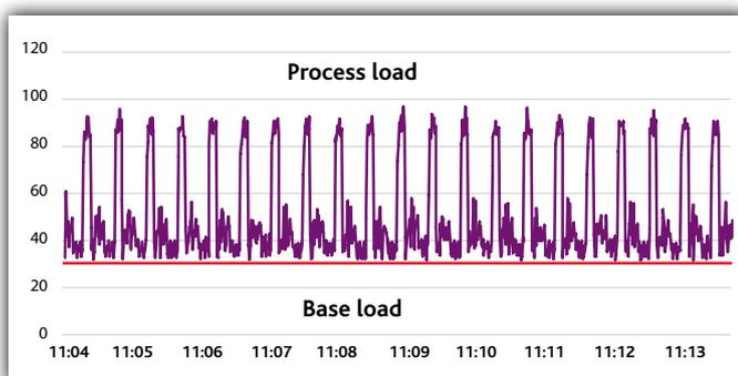
*Figure 3: This expanded view of injection machine power draw shows detailed cycle stages*
