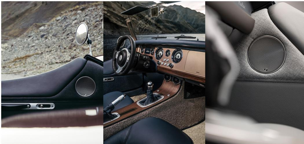
The system includes eight transducers: four conventional speakers in the door and rear panel, and four invisible speakers, of which three are behind the dashboard and one in the lower compartment panel for bass reproduction. The transducers are controlled by a new amplifier with a dedicated DSP, powered by Sennheiser's audio processing software.
