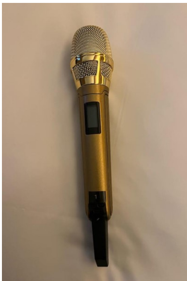
Brandi Carlile’s Sennheiser SKM 6000 handheld transmitter with Neumann KK 205 microphone capsule, plated in gold
