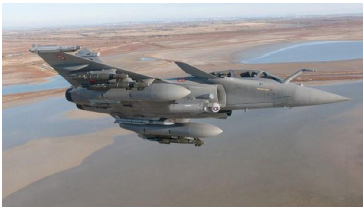
Rafale B with six AASM missiles, two MICA IRs (outer hardpoints), two Meteors (side, rear), two 2,000-litre external fuel tanks and one Talios pod. © Dassault Aviation - A. Pecchi
