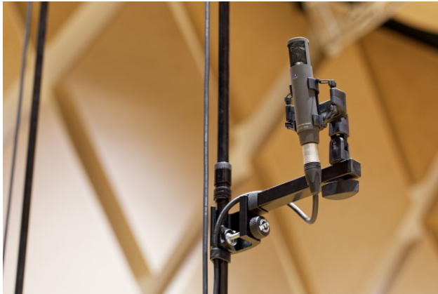
The Sennheiser MKH 800 TWIN is equipped with a dual capsule and provides two separate output signals
