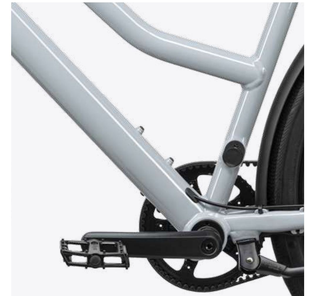
Integrated battery in the downtube
