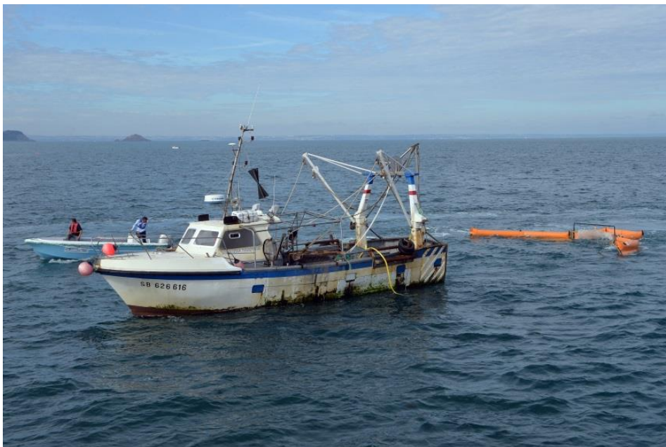
Fishing boat fitted with special trawl which collects 6-8 tonnes of floating litter [Image taken at WFO event in Kerval, France July 2016]
