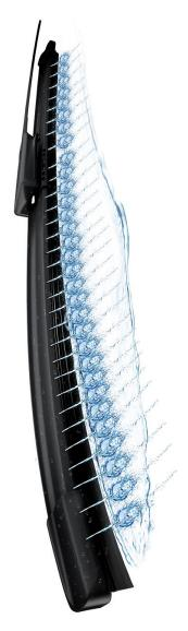
Valeo's new patented wiper technology, Valeo AquaBlade™ (integrated in the Valeo Silencio™ wiper range) delivers wiper fluid directly onto the windshield via the wiper blades, rather than via nozzles mounted on the hood. The windshield is wiped instantly and uniformly, regardless of vehicle speed, allowing for constant and perfect visibility. Front-facing cameras, which are now more and more common on car windshields, also benefit from an improved field of vision.
