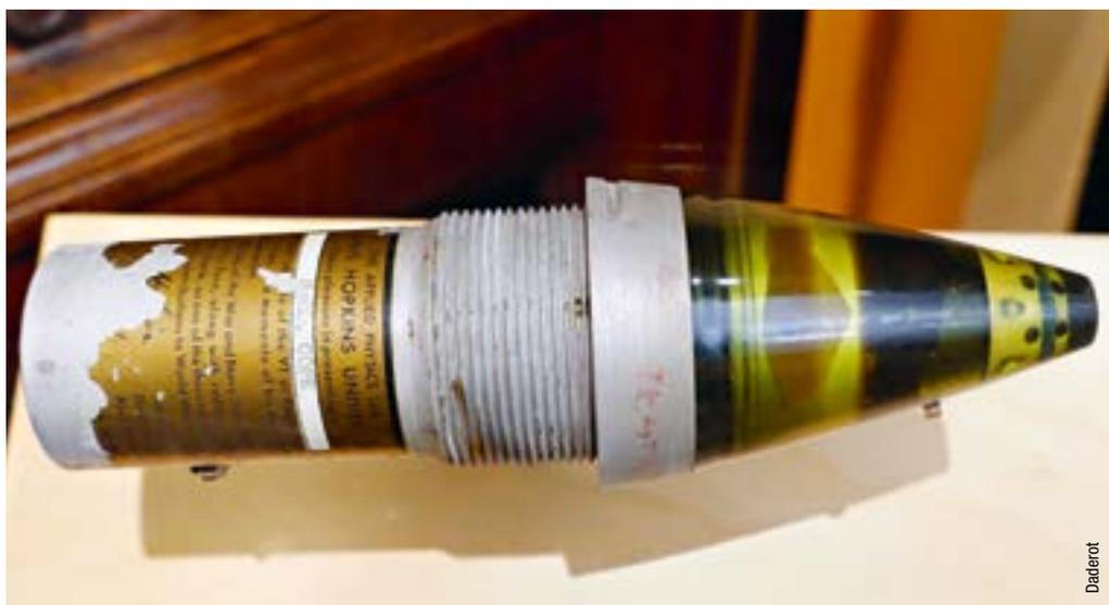
A proximity fuze is designed to detonate automatically at a specific distance from the target.
