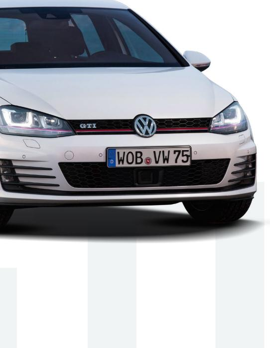
Golf GTI Mk7. The seventh generation of the GTI was launched in two output versions in 2012. The base version delivered 162 kW/220 PS while the Golf GTI Performance could unleash 169 kW/230 PS. Equipped with a new front differential lock, the Performance version masterfully redefined traction for front-wheel drive vehicles.
