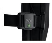
The triggering unit, which is fixed permanently to the airbag, includes a battery, memory chips and interfaces (USB/Bluetooth). Its overall weight, including the airbag is approximately 800 q. The mechanical deployment is implemented via the activation of an e-igniter. This builds up stagnation pressure that drives a needle through the sealing cap of the compressed-gas cylinder. Under atmospheric pressure, the liquid CO2 expands and fills the airbag within milliseconds.
