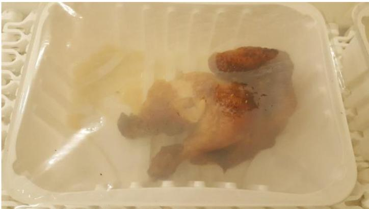
CIRCPACK tray sealed for barrier test
