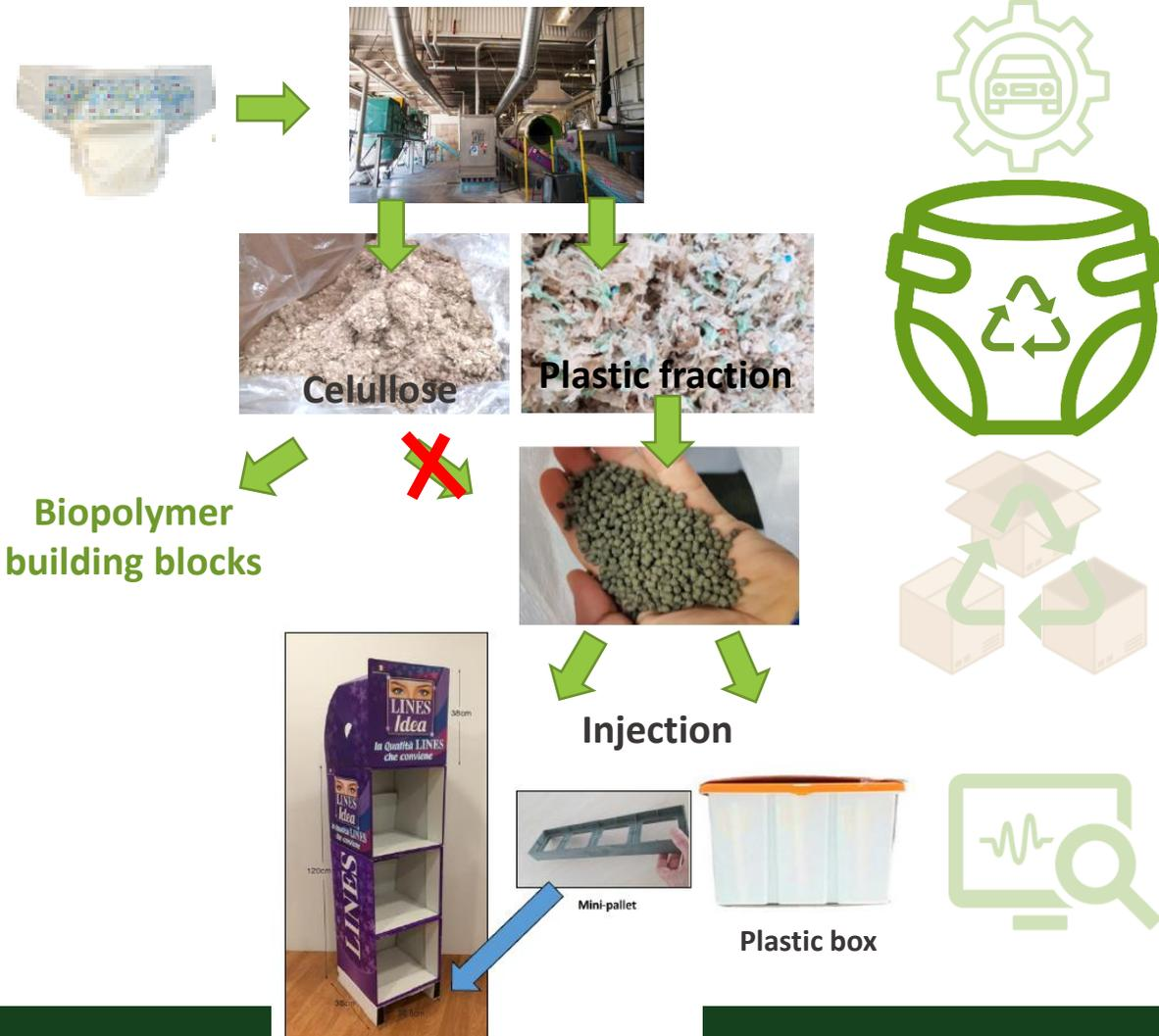
Plant upgraded. Fractions successfully separated and improved quality (plastic, cellulose, SAP)
