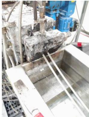
Extrusion of PE
