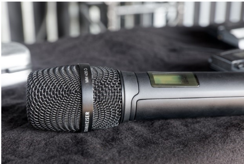
Sennheiser MM 435 microphone head with a dynamic high-end capsule (cardioid)
