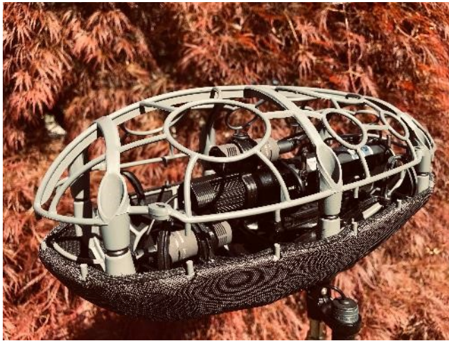
A view inside the blimp: Thomas Rex Beverly's double mid-side microphone configuration consists of two Sennheiser MKH 8040s and an MKH 30
