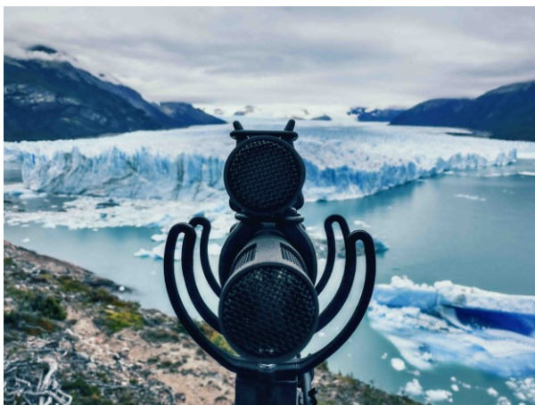
Beverly tried the new MKH 8030 in an MS configuration with the MKH 8040 (photo taken at Moreno Glacier)
