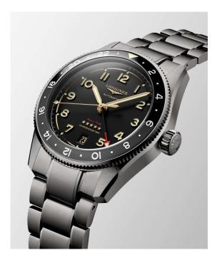
The model is powered by the exclusive Longines GMT calibre L844.4, equipped with a silicon balance-spring and innovative components, offering a resistance to magnetic fields ten times greater than the ISO 764 reference standard. This extremely precise self-winding mechanical movement has a power reserve of up to 72 hours. It is officially certified as a chronometer by the COSC (Contrôle Officiel Suisse des Chronomètres).
