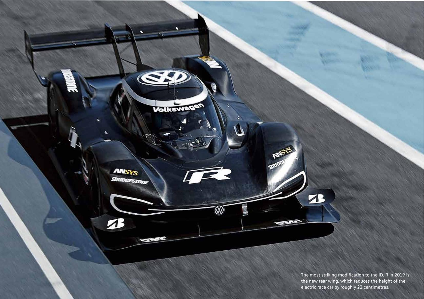
The most striking modification to the ID. R in 2019 is the new rear wing, which reduces the height of the electric race car by roughly 22 centimetres.
