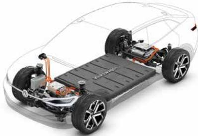
All the cars in the ID. family are based on the new MEB platform (modular electric drive matrix).
