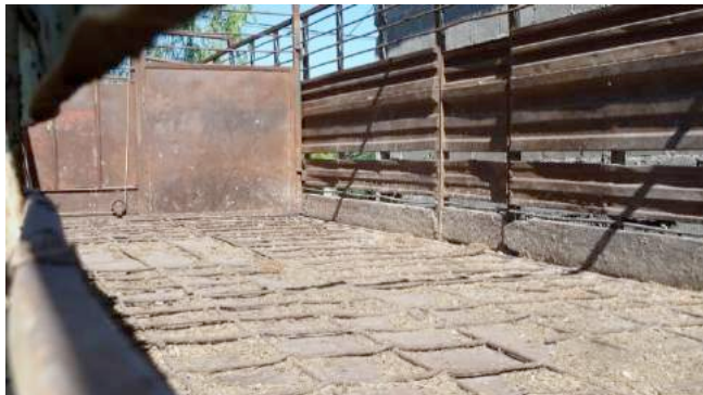
Bardanca's rusty trailer with sharp-edged slits.
