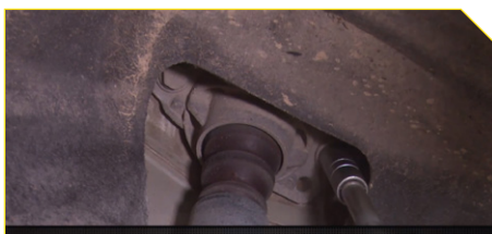
4. Unscrew the indicated screws of the top mount
