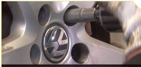
2. Disassemble the rear wheel
