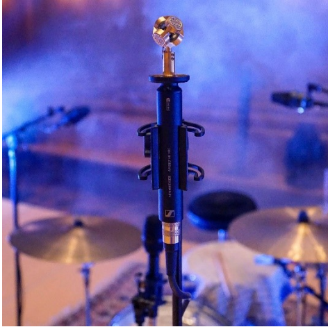
The AMBEO VR Mic – pictured without the mic basket – is an ideal tool for providing the 3D audio basis in immersive audio productions
