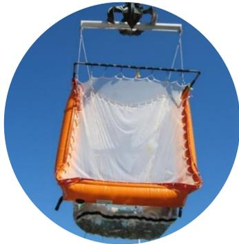
Fishing boats are fitted with **trawls which collect between 2-8 tonnes marine litter** for cleaning and recycling.
