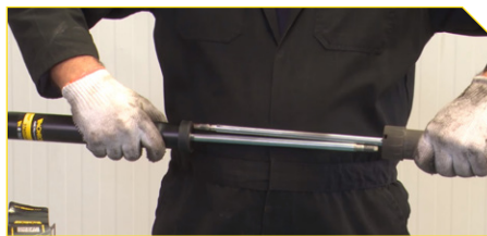
7. Compare the old shock absorber to the new one to be sure it fits
