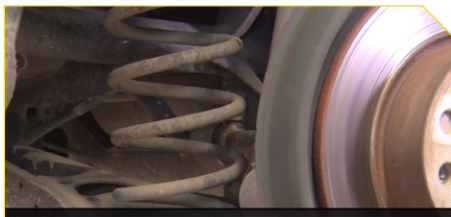
3. Use hydraulic jack to keep rear spring compressed
