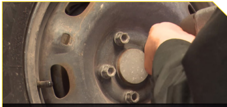
2. Disassemble the rear wheel
