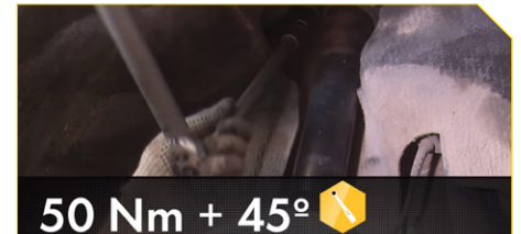
9. Fit the shock absorber to the car body by tightening the top mounting nuts to 50Nm + 45°
