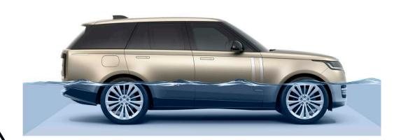
\*Wading depth (25 deg entry and exit) 750mm, Deep Fording depth (9 deg entry and exit) 900mm.
