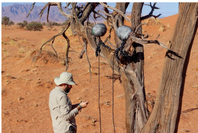
George’s favourite recording rig employs four MKH 8020s placed around a tree – a head-related recording
