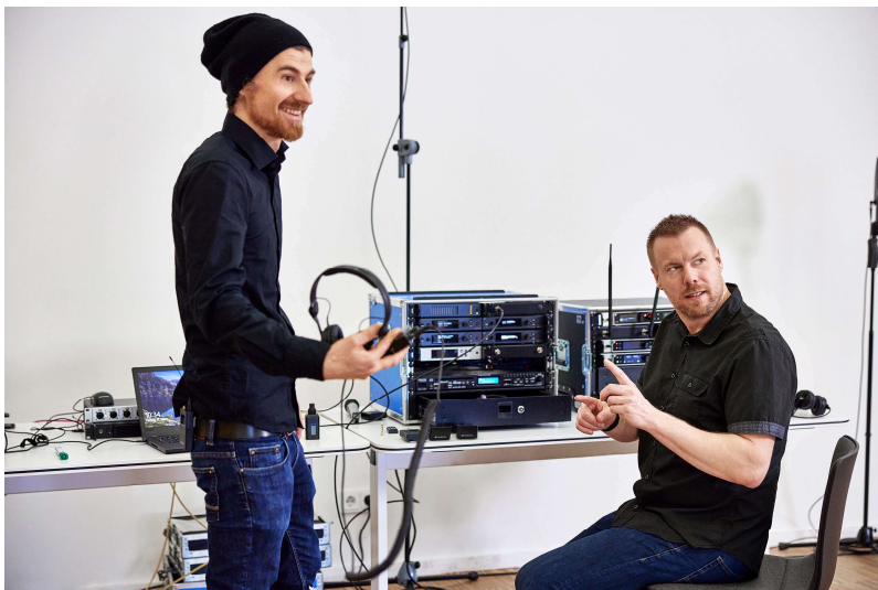
Marco and Jonas with the RF equipment. Narrowband IEM transmitters and mic receivers centre and right; the 1U, 19” WMAS prototype on the left
